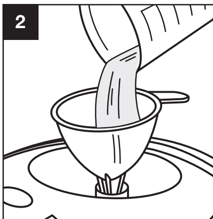
2 Fill the tank using the funnel and measuring cup provided. The tank holds up to 40 oz. /1200ml of water. DO NOT overfill the water tank or damage to the product may occur.
